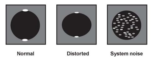
Measure the dimensions of the 4 mm cystic target to check the image geometry. Use the calipers to measure from top to bottom and side to side. Repeat with the other cystic target groups as part of the cyst imaging test.
